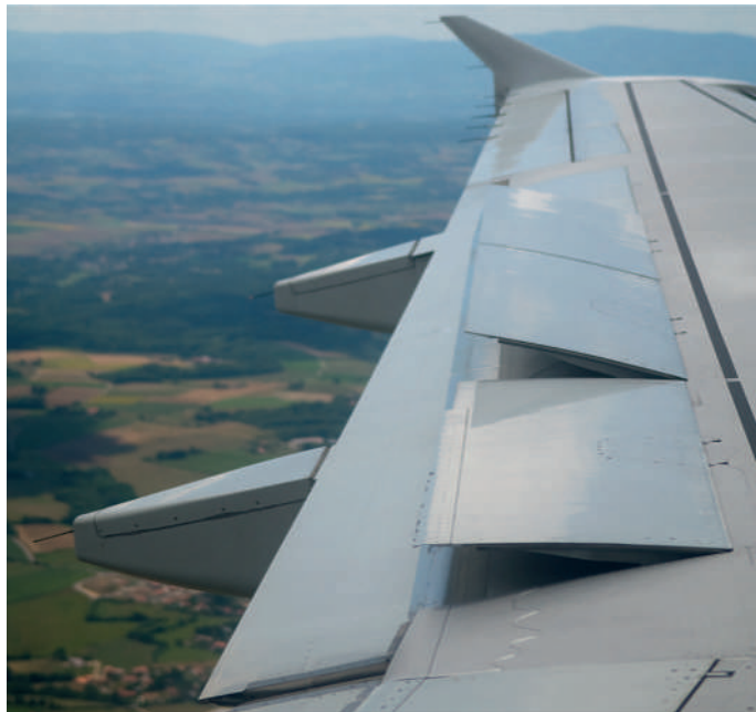
35 Application example, brake flap drive on aircraft wing
