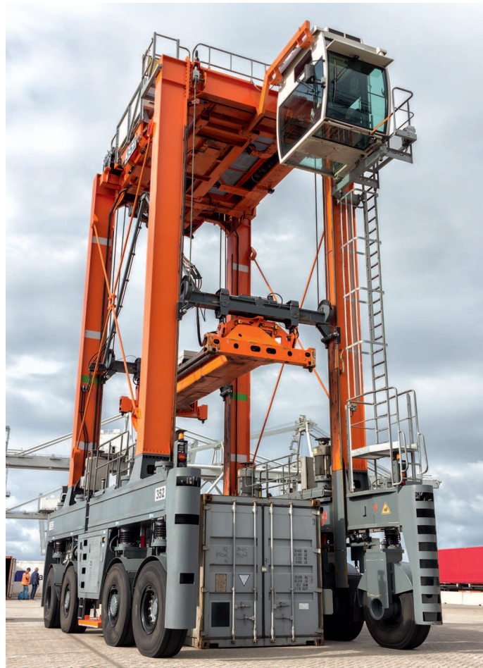
④23 Application example, straddle truck
